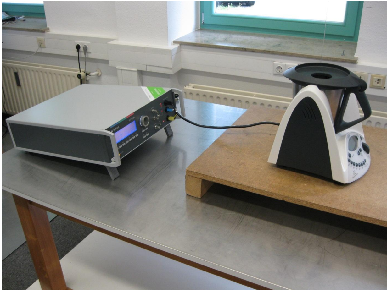
Burst to AC supply lines EUT on insulated support distance generator to EUT =0.5m
